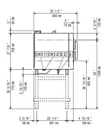
CWII Cold Water inlet 1 CWI2 Cold Water Inlet 2 FΙ Electrical inlet (power) G Gas connection
